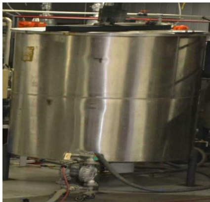
Figure 6. Exemplar AB Specialty batch tank with agitator and lid (CSB investigation team., 2021)
